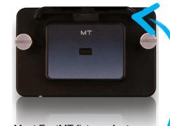
Most FastMT fixtures feature a zero insertion force toggle at the top, pressed using either the left or right hand. Once the toggle is released, a spring mechanism holds the connector snugly in place, providing stability for clear, in-focus imaging of the ferrule and fibers.
